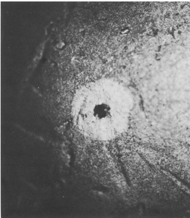
Figure 9 Micro-pit in AISI 440C rolling element, \times 30 .
